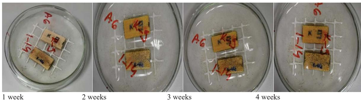
Figure 3. Pictures of samples exposed to *A. niger*.
