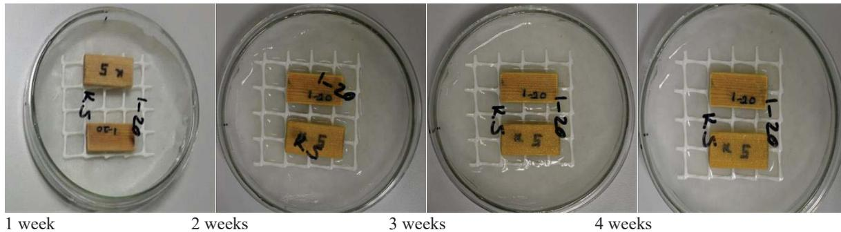
Figure 2. Pictures of samples exposed to *P. chrysogenum*.
