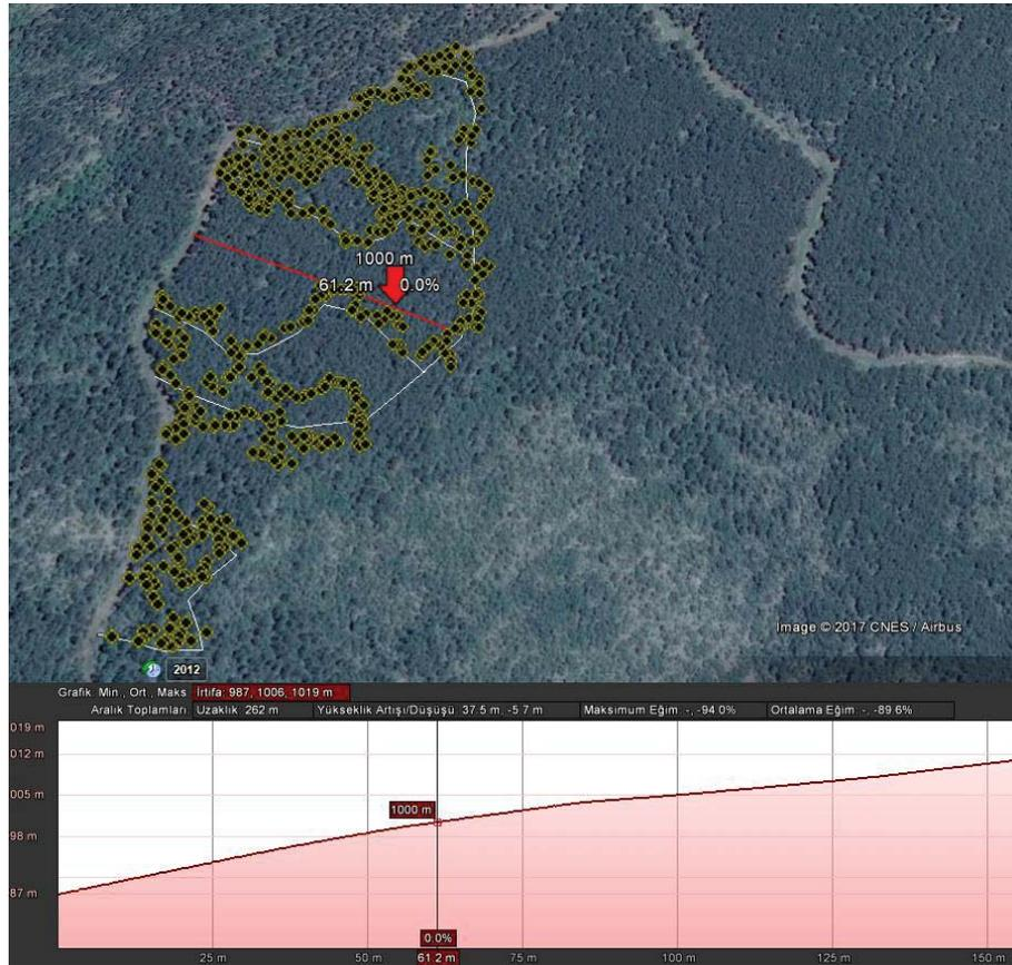
Figure 8. Slope evaluation of possible skid trails
